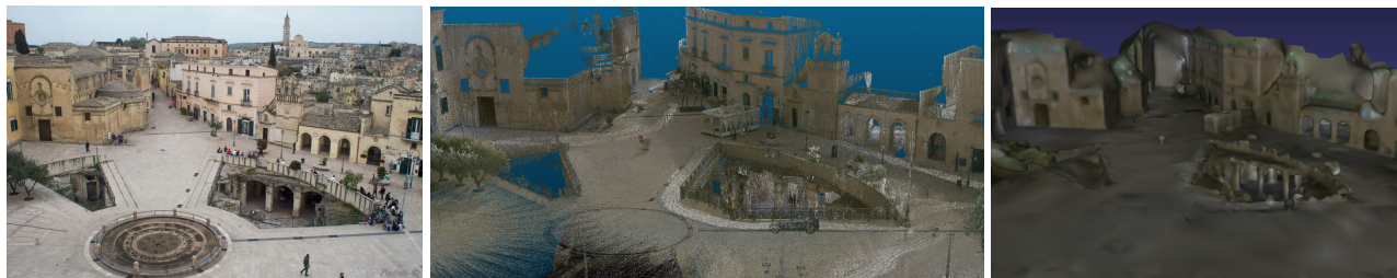
Figure 1: Left: view of the Vittorio Veneto square (the hypogeum is underneath). Middle: Acquired points cloud. Right: Reconstructed triangle mesh.
