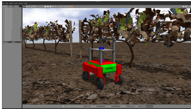
Figure 2: The simulated environment developed in Gazebo composed by a vineyard row and the digital twin of the robotic platform equipped with several sensors.
