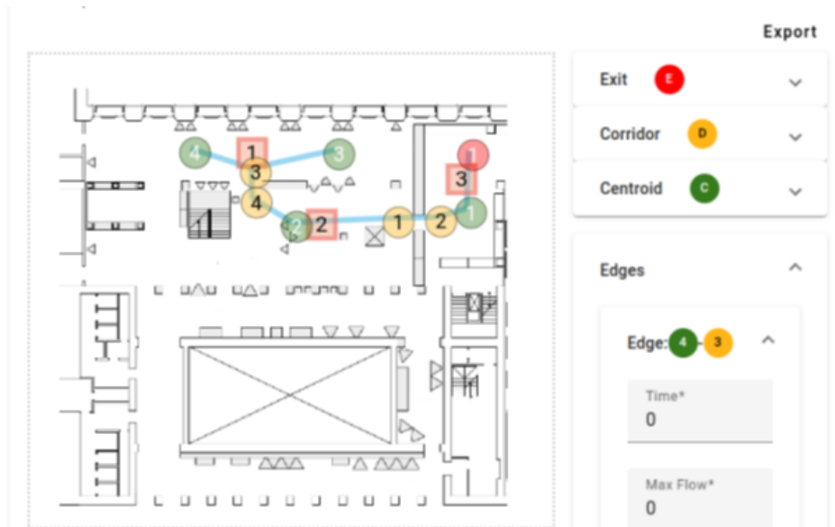
Figure 1: Screenshot of the ECV-Suite web app with details of the graph modeling the museum planimetry.
